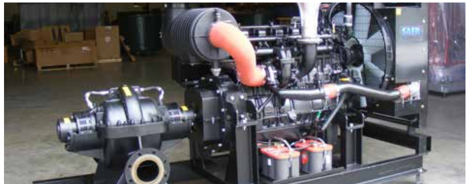
NR. 2 SKDZ 125-335 WITH DIESEL ENGINE SPAIN MOBILE FIREFIGHTING SYSTEM
